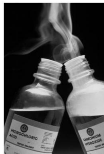
Figure 3. Reaction of hydrogen chloride with ammonia
