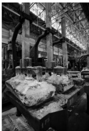
Figure 5. Electrolysis of aluminium oxide
