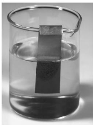
Figure 2. Reaction of zinc metal with a solution of copper(II) sulfate
